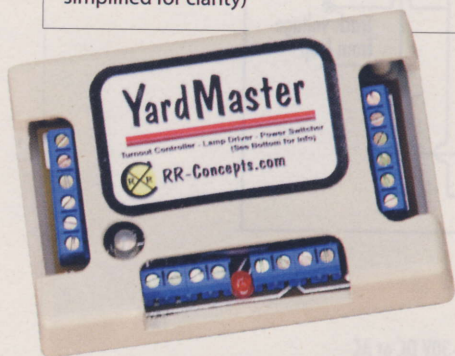
Figure 7: Railroad Concepts “YardMaster” (Connections to sensors and switch machines simplified for clarity)
